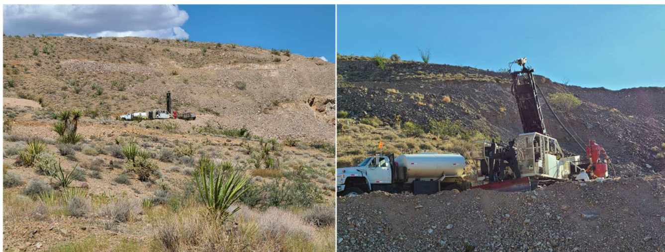
Figure 2. Left, drill rig set up on the Excelsior Zone. Right, close up of track mounted drill rig drilling hole GR21-50.
