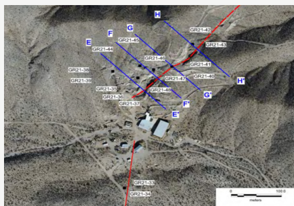
First pass test covers 350m of strike and 50 to 100m vertical
