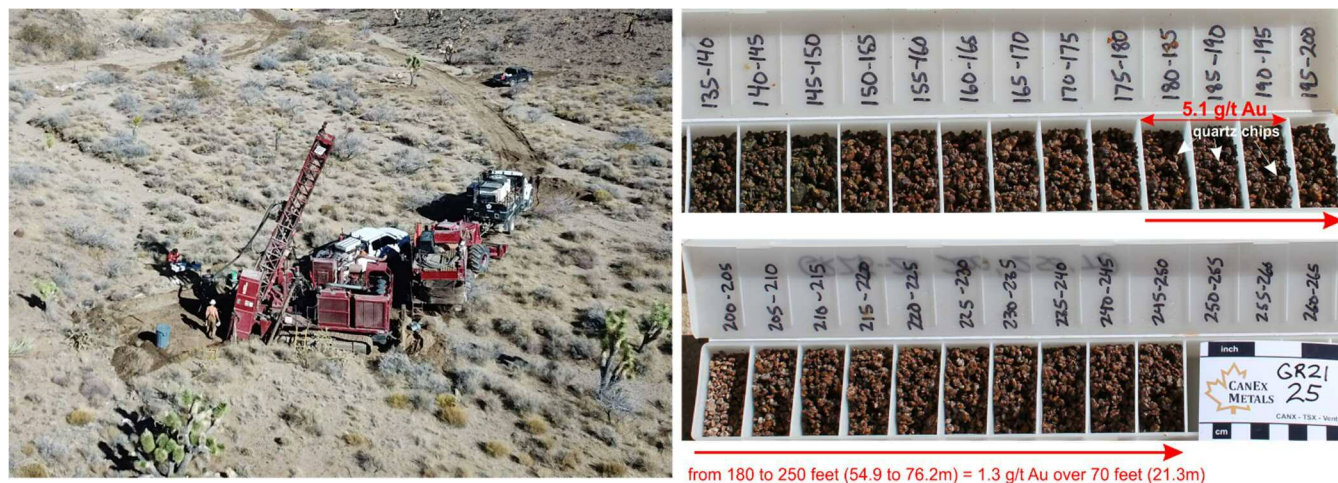
Figure 1. Left, RC drilling at the Eldorado Zone. Right, Reverse circulation drill chips collected from hole GR21-25 showing the lower mineralized interval. Note the highly oxidized red hematite-stained nature of the rock chips containing fragments of quartz throughout the mineralized interval.
