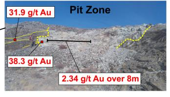
Exposed mineralization at the Pit Zone (white dotted lines) strongly correlates with an analytical signal magnetic low which suggests the zone is open to the northwest and could be at least 450 metres long. The magnetic low is interpreted to represent hydothermal alteration and magnetite destruction within the highly magnetic orthogneiss host rock
